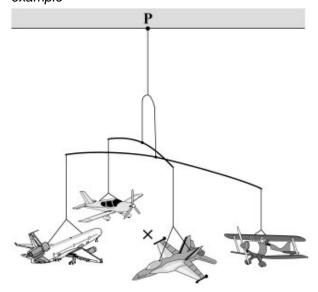
(ii) the centre of mass is (vertically) below the point of suspension / P
