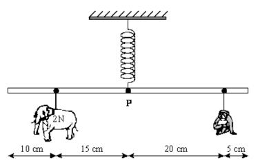
(i) Use the following equation to calculate the moment exerted by the elephant shape of weight 2N about the pivot **P**. Show clearly how you work out your answer and give the unit.
