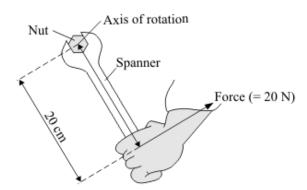
Use the equation in the box to calculate the spanner's turning effect in newton metres.
