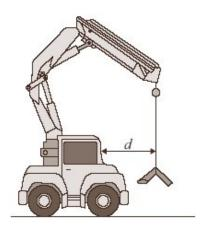
The distance, d, is measured to the front of the cab.
