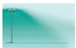
Within the overall distribution of radio waves from a base station across its cell, there is a zone where the concentration is higher than elsewhere.
